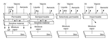
13.6 Types of CB protective materials. LP, low hydrostatic pressure; HP, high hydrostatic pressure.
